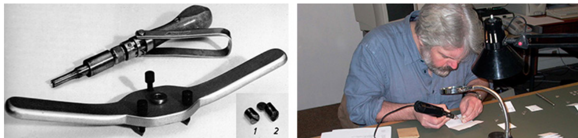
Figure 21 (left) Core cutter [26] and (right) core drilling [14].
