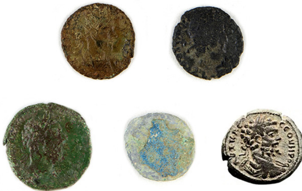
Figure 13 Examples of different kinds of patina aesthetics on copper-based roman coins, from top left to bottom right: cuprite red (ID 587202), tenorite black (ID 570103/1), malachite green (ID 579679), azurite blue (ID 20.S239-2.2569) and silicate “desert” [40] patinas. Coin images are not to scale. Coins 587202, 570103/1 and 579679 are reproduced upon permission of the Ministry of Culture, Regional Directorate of Museums of Friuli Venezia Giulia. Coin 20.S239-2.2569 is reproduced upon permission of the Ministry of Culture, General Directorate of Archaeology, Fine Arts and Landscape of Friuli Venezia Giulia. Any further reproduction of such images, duplication by any means, as well as downloading and subsequent manipulation, is strictly prohibited.
