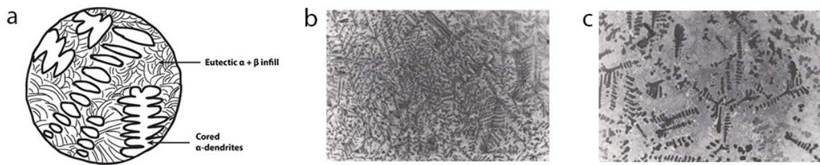
Figure 9 a) Schematic example of a Cu-Ag eutectic structure. b-c) Micrographic example of a 40% Cu - 60% Ag alloy. α dendrites and α + β eutectic infill are clearly visible ([27], original magnification: x35 (b), x100 (c), © 1991 J. Paul Getty Trust).
