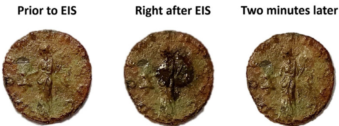
Figure 99 Visual evaluation of the invasivity of the EIS measurements conducted on coin 587202. For reference, the max diameter of the coin is 16 mm. Reproduced upon permission of the Ministry of Culture, Regional Directorate of Museums of
