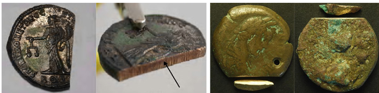
Figure 20 How sampling can visually impact on coins [81,82]. Both coins in figure have been cut in order to allow the investigation of their bulk and of their corrosion layers, at a high cost in terms of aesthetic impact on the sample. The black arrow points toward the cut side. Image on the left is reprinted from [82], with permission from Elsevier.
